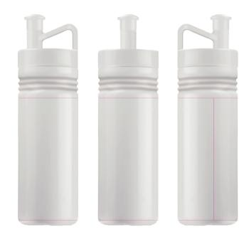
NOTE - THE SEAM LINE COULD AFFECT ON IMPRINT - BREAK OR CONVEXITY
